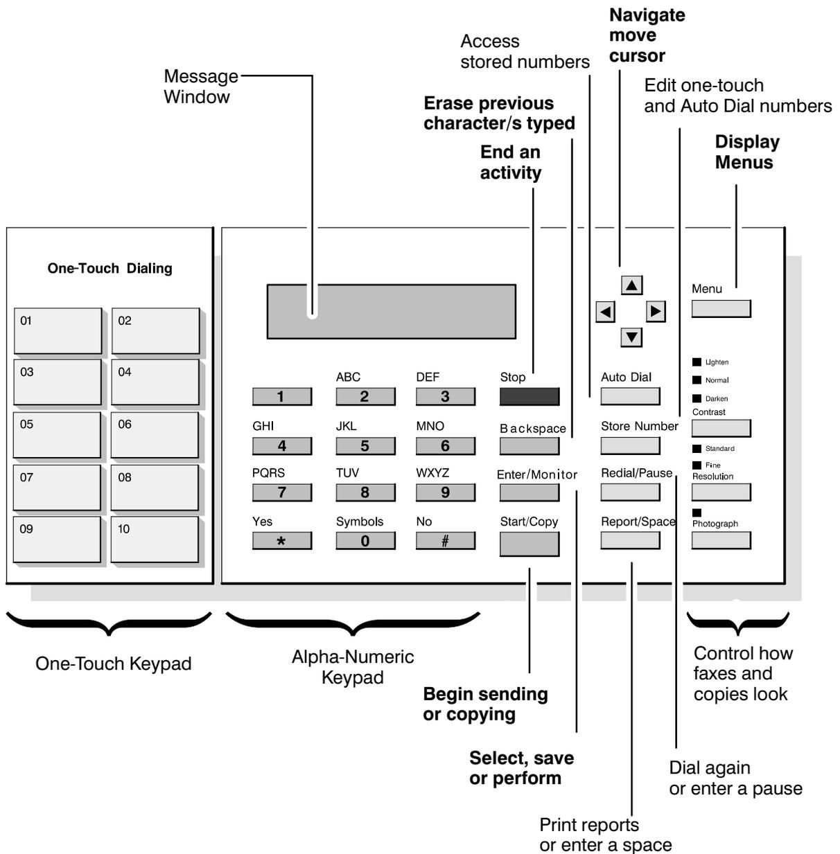
Figure 3-1. Control Panel (HP FAX-700 and HP FAX-750)
