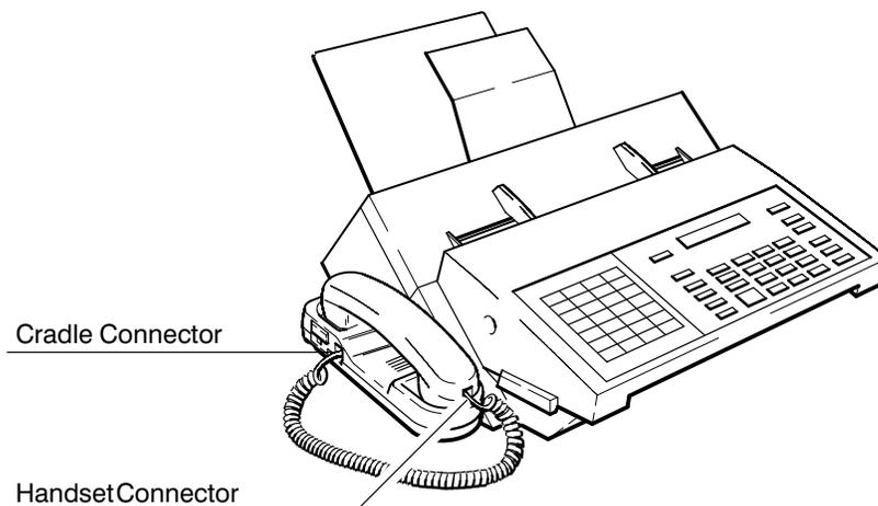
**Figure 2-37. Installing the Handset in the HP FAX-950**
