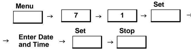
**Note** Your fax machine is equipped with a Daylight Savings Time feature. This means that the fax machine clock will automatically set the time forward 1 hour on the first Sunday in April (that is, 2:00 am to 3:00 am) and set the time back one hour the last Sunday in October (that is, 2:00 am to 1:00 am). If you do not want this feature enabled, you need to change fax parameter 35 to the Invalid setting. Fax parameters are presented in chapter 4 of this guide.
