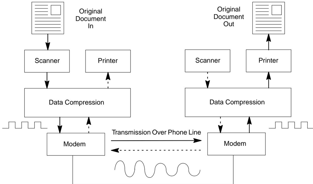
**Figure 1-1. Simple Diagram of Transmission Between Fax Machines**
